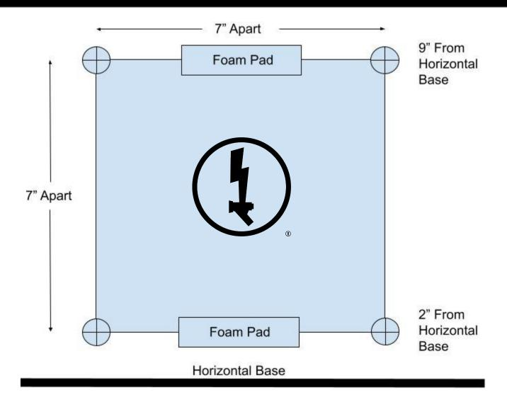
\*This is a diagram depicting the recommended placement of the stainless steel D-rings for mounting your QuikTap® Tabletop Dispenser on a supported, horizontal surface such as a golf beverage cart. It is recommended that you use the proper mounting screws based on the substrate of which you will be drilling/screwing into. This diagram is **NOT TO SCALE** and is not intended to be a template.
